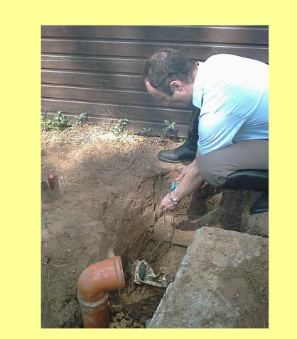
2. Active sub-surface sampling: Active sampling by the same method as for surface sampling but with connection of a sampling probe: the stainless steel tube has an internal diameter of 1cm and a total length of 130cm. An additional connection can be added to increase the sampling depth (up to a total length of 3m).
