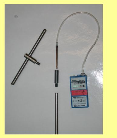
3. Sampling probe: The end of the probe can be drilled in the soil without
